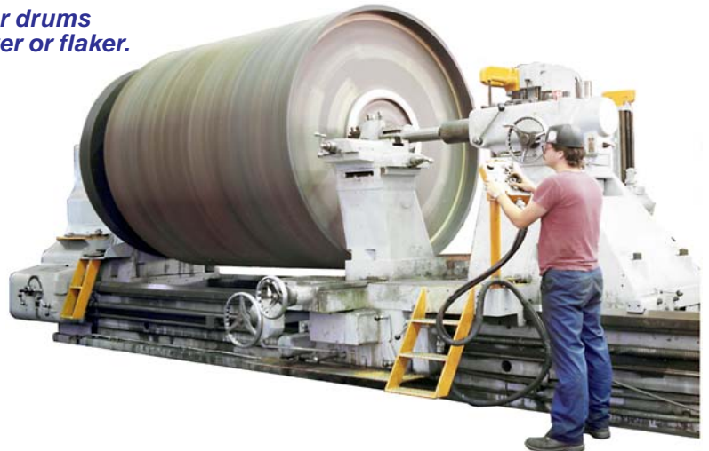
drum surface & trunnion repair
